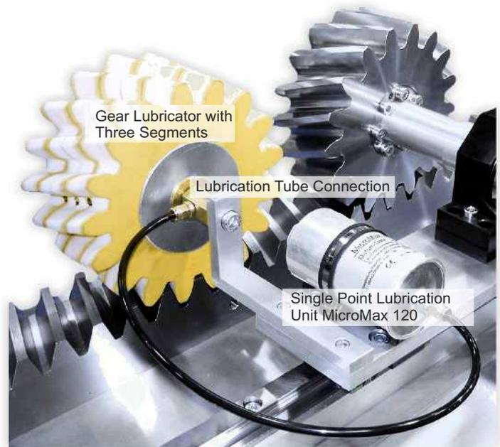
The LUBCON LubeGearSystem can be operated in combination with a single point lubrication unit or a central lubrication system. In comparison to manual lubrication, LUBCON LubeGearSystem is a cost efficient, easy and effective solution for smooth lubricant application.
