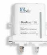
Double point lubrication unit for maintenance-free operation of e. g. electric motors up to a maximum of 3 years. It can also be used for fan shaft bearings and many others with a large variety of long life greases.
